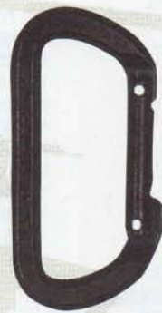
277 BLACK D CARABINER , 105mm, high strength aluminum alloy, 4 1/4" size, 5500 lb test, black anodized finish
