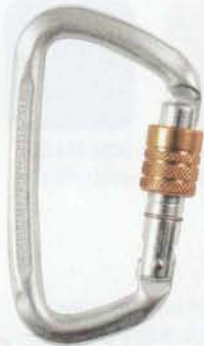
163 HARD STEEL MODIFIED D KEY SCREW GATE CARABINER , 6.6 oz., 105mm, 21mm gate opening, 11,250 lb test, rating stamped on each unit
