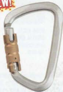
248 HARD STEEL LARGE D KEY STAGE 3 AUTO LOCK CARABINER , heat hardened & nickel plated for ultimate strength & durability, 20mm gate opening, 11,240 lb test, rating stamped on each unit, CE certified
